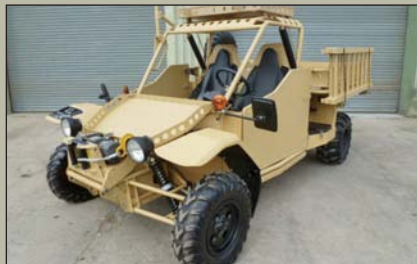
EPS Springer ATV LHD 1.1 ton payload, 2 seater left hand drive configuration, 4x2, fitted Lombardini 1.4 litre diesel engine and 2 speed forward and 2 reverse CVT, 1.4 litre Lombardini diesel engine, etc, Year 2009, Mileage from 100 kms, Excellent Condition, Price £10,500 (75 Available)
