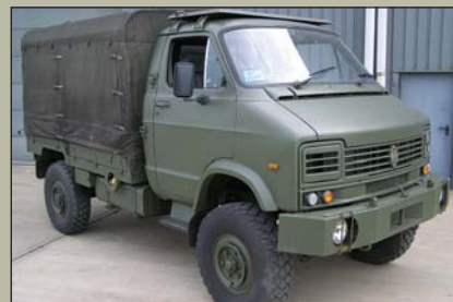
Reynolds Boughton RB 44 Truck Cab Pickup R.H.D, Permanent 4x4, 5 speed g/box, hi/lo box differential Lock, power steering, carries 2250 kgs, Perkins Phaser 110T T/Diesel engine, Mileage from 37,000, Guide price from £3,750 (10 Available)
